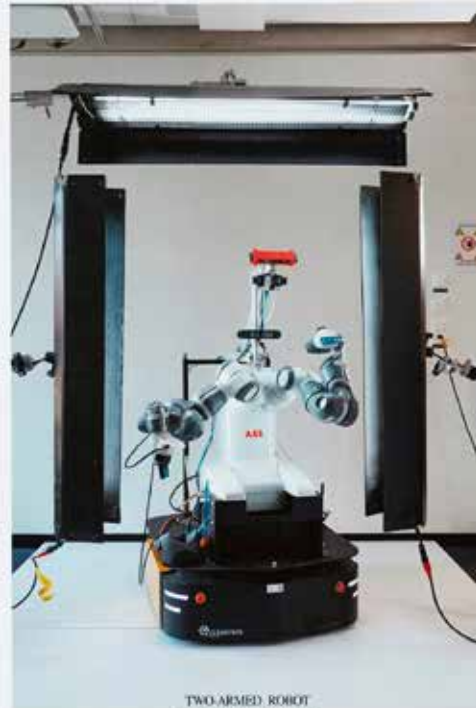
TWO-ARMED ROBOT on a mobile platform. It is able to move independently, detect objects, grasp them, and manipulate them.
